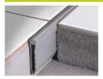
COFLEX CF mortar bed movement joints in co-extruded synthetic resin are conceived to subdivide large tile bays. Exclusively suitable for pedestrian traffic, this profile provides limited protection to the tile edges and compensates slight differential movement due to substrate contraction and expansion. They are installed with thin-set mortar. Ideally used in retail shops, hotels, sports facilities and schools
